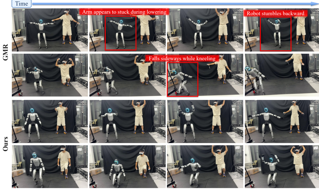
Figure 6: Streaming Unitree G1 teleoperation driven by GMR (top two rows) and SMR (bottom two rows) through MimicLite. Each row shows four frames from an independent recording in temporal order, covering arm motion or kneeling.
