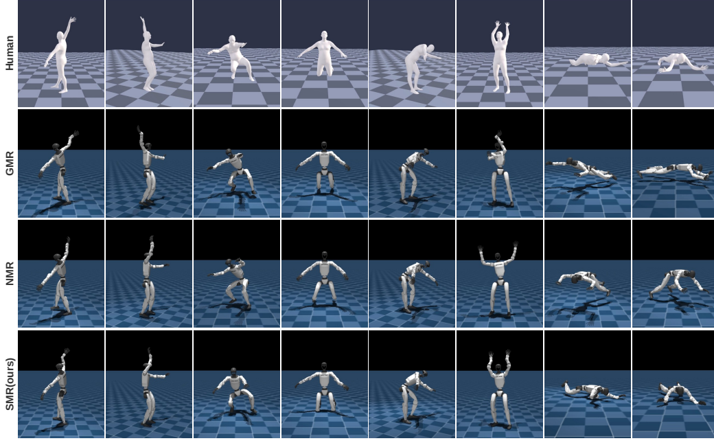
Figure 3: Qualitative comparison of Unitree G1 reference poses at matched timestamps from eight human motions. The rows show source SMPL poses and the corresponding references produced by GMR, NMR, and SMR. Compared with GMR and NMR, SMR better preserves the source whole-body posture, especially in the crouching, kneeling, and floor-level examples.
